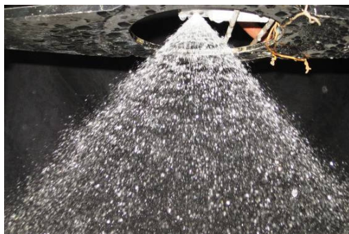
Figure 17. Fully Opened Spray Cone Under design condition ( P_f=10 , P_o=4 bar)
