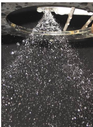
Figure 19. Spray cone angle of external nozzle
