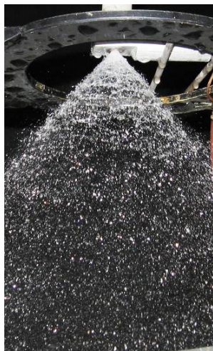
Figure 18. Spray cone angle of internal nozzle
