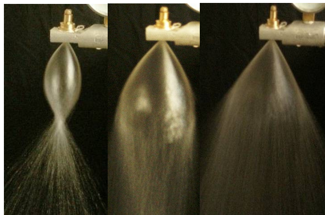
Figure 16. Spray Formation Stages with Regarding to Fluid Swirl
