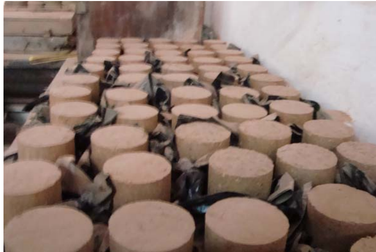
Figure 1. Tropical reddish-brown soil specimens on the drying table
