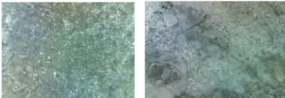
Figure 4a (left) and 4b (right). Micrograph of the film deposited from \text{AgNO}_3 and \text{NaCN} solution on zinc and lead metallic substrates respectively
