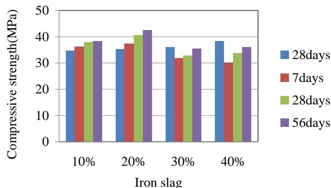
**Figure 3.** Compressive Strength after immersion in Mg SO<sub>4</sub> solution (50g/l)
