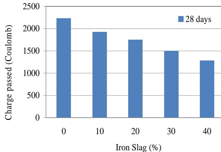
**Figure 4.** Rapid Chloride Permeability Test
