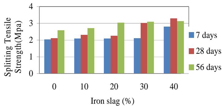
**Figure 2.** Splitting Tensile Strength of Mortar
