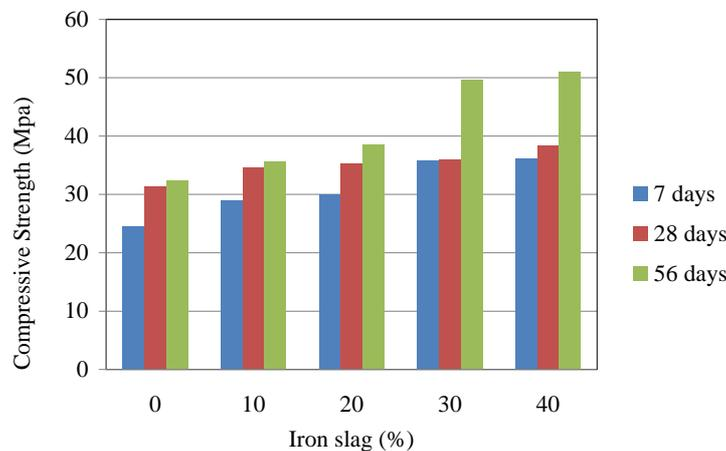
**Figure 1.** *Compressive Strength of Mortar*
