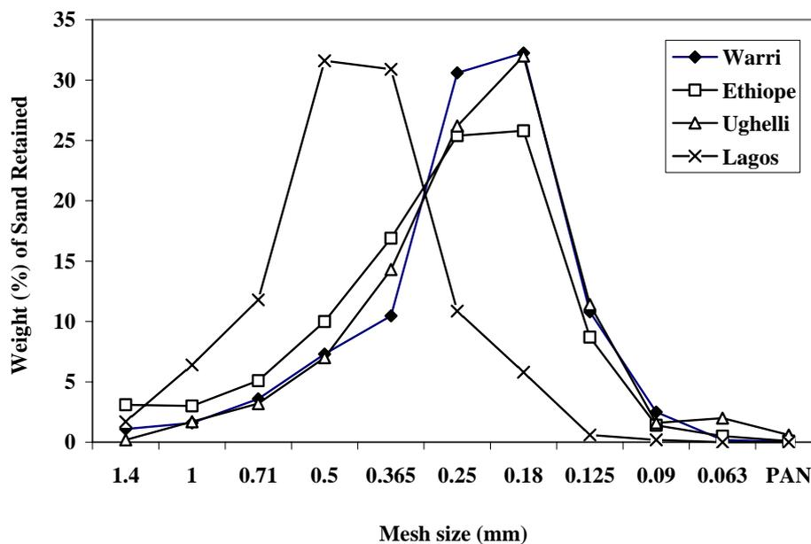
Figure 1. Grain size distribution curves
