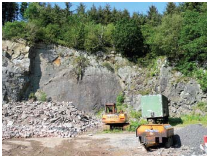
Figure 2. Working face of a crushed stone operation showing rubble created by blasting [11]
