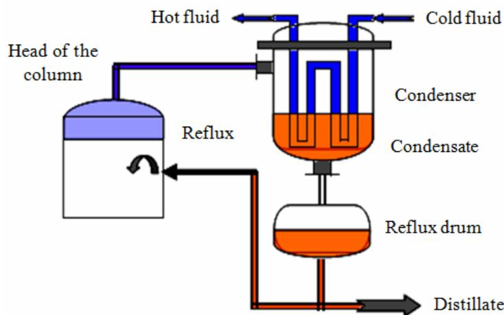
***Figure 1. The condenser operating in the distillation column***
