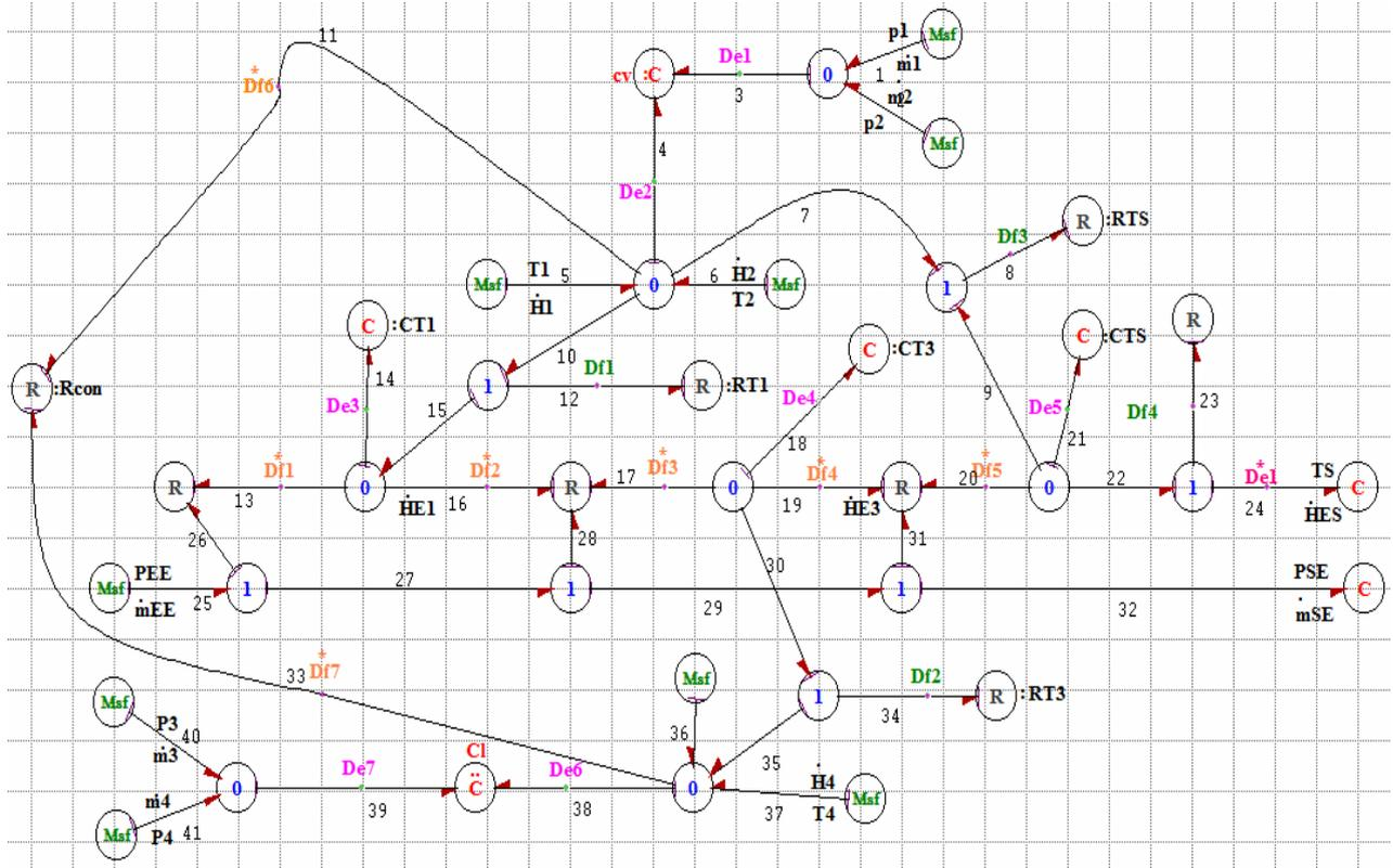
Figure 2. Bond graph model of the condenser with sensors placement
