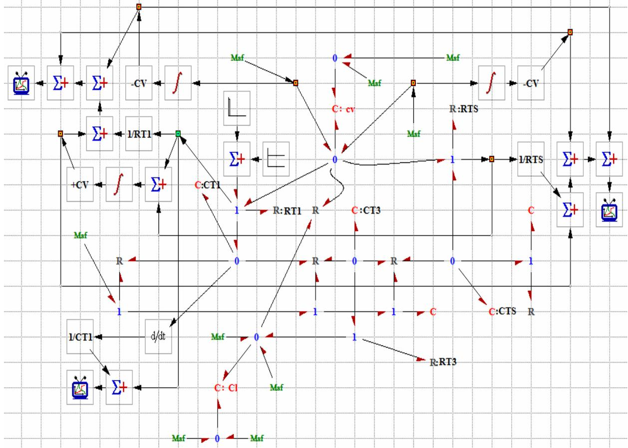
Figure 3. Block diagram representing the ARR1 function of  $Df_1$
