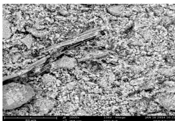
Figure 3. Micrograph of H 2 SO 4 modified clay
