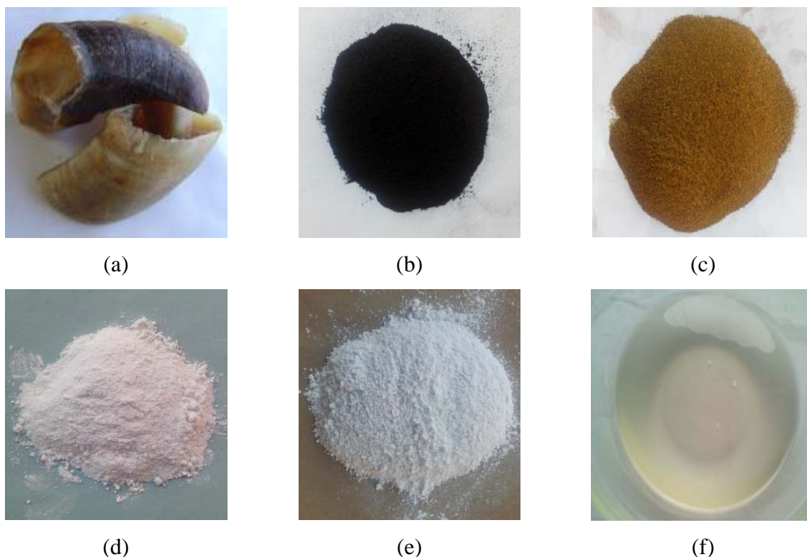
Figure 1. Photographs of the selected materials: (a) Unpulverized cow hooves, (b) Graphite, (c) Pulverised cow hooves, (d) Barium sulphate, (e) Aluminium oxide, (f) Epoxy resin
