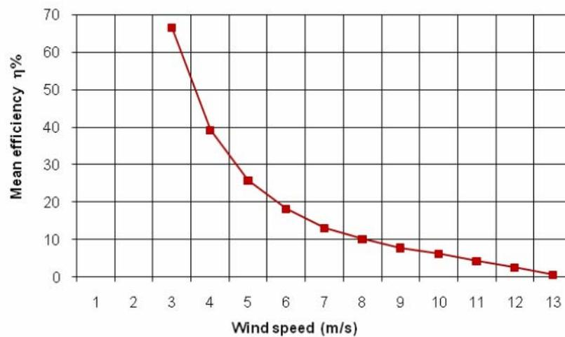
Figure 11. Mean efficiency of system in function of the wind speed
