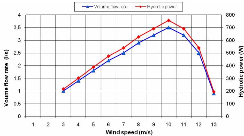
Figure 9. Variation curves of the water flow and the hydraulic power
