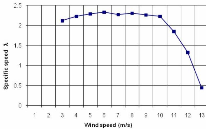
Figure 10. Specific speed of rotor in function of the wind speed
