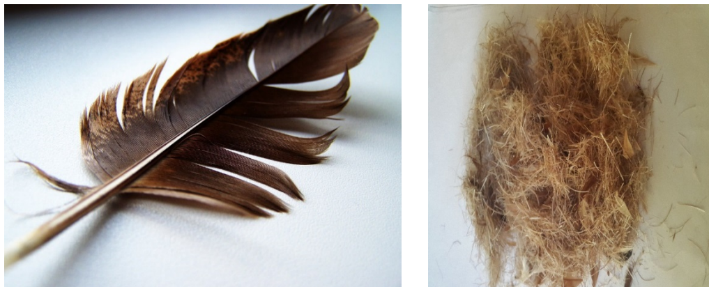
Figure 1. (a) and (b) illustrate the brown chicken feather and the extracted CFF
