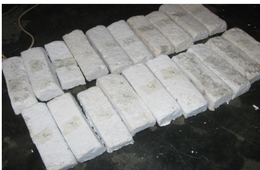
Figure 3. Samples prepared for flexural test
